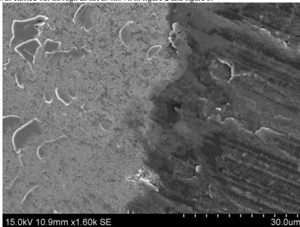
Figure 2 Wear morphology of the flank face
